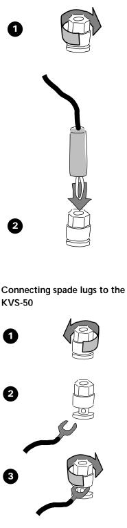
If the lug is too narrow, insert one prong through the hole in the post, making sure that the positive and negative prongs don't touch each other.
